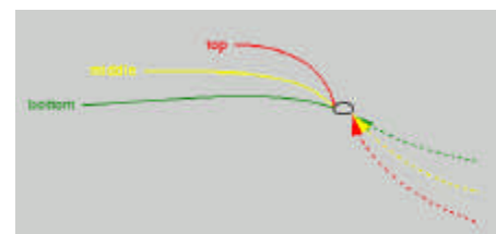
Effect of twisted apparent wind and upwash on sail's twist.
