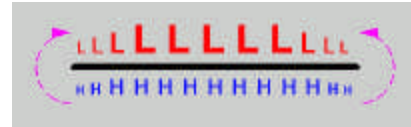
Rear view of a wing showing formation of wingtip vortices as air flows from high pressure below to low pressure above.
